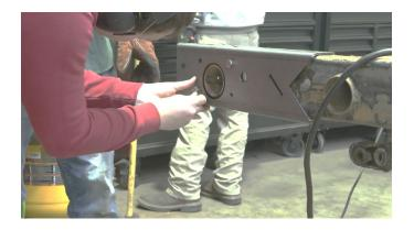
Once the tac weld is complete, be sure to weld 100% around all edges to prevent exposure to moisture and protect against future corrosion.
