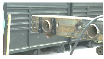
Additionally, grind the frame rails free of rust to expose the bare metal where your repair section will be installed.
