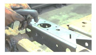
Hold the center frame section up to the frame making sure the frame holes align. If they do, insert two bolts to secure the component in a fixed position.
