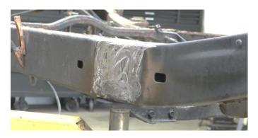
Spray the work area with a weld through primer to help prevent or reduce the risk of rust formation.
