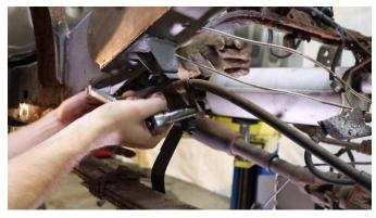
Hold the part up to the frame and take note of its coverage. Mark off any sections you wish to cut off, while leaving enough to weld back on to.
