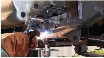
The inner wall of the part features a perforation that can bend into the channel. Before finalizing the weld, use c-clamps to close the gap. This may require further cleaning of the frame to install.
