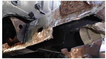
Push the part into place, using the angle and brackets for alignment.
