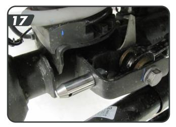
ao. Install the longer disconnect post on the driver side axle sway bar link mount with it pointing inboard [18]. Fasten with the ½" nylock nut and tighten to 64 ft-lbs. Tighten the post with the pin hole parallel to the ground. Slide the polyurethane spacer on the pin up against the axle tab.
