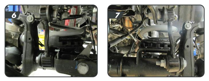
h. Remove the 4 bolts mounting the front driveshaft to the pinion flange (15mm). This is done to ensure the driveshaft does not bind when removing the coil springs. [8]
