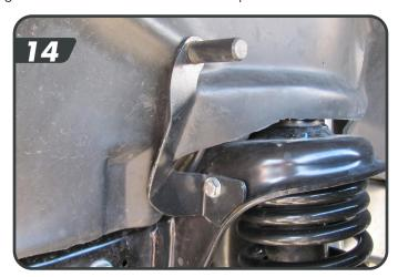
JT Mojave models with JKS9613: Install two provided ¼" donut spacers (01499) between the reservoir hose retaining wire and frame using the OE bolt [15] and tighten to 6 ft-lbs (first mount forwards of the coil spring). Verify reservoir hose clearance to the disconnect retention bracket once installed.
