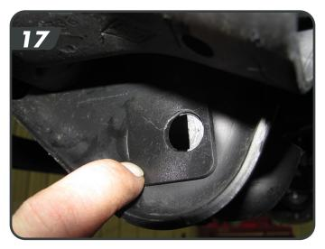
d. Re-install the control arm to the axle with the factory bolt with cam lock washers. Rotate the cam lock so that the bolt will be as far back in the slot as possible (most rearward setting = max caster). Snug the cam hardware so that the cams are retained within the stops. Final torque will be completed with the weight of the vehicle on the suspension. [18]
