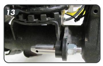
The kit comes with disconnect retention brackets to hold the links when the links are disconnected. Install the retention brackets using the provided 5/16" bolts into the factory hole in the front of the coil bucket [14]. These are designed to slightly interfere with the edge of the coil bucket to hold them in place.
