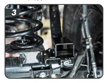
The shocks come with the bushings and upper spacers pre-installed. JSPEC shocks will be installed body down, Fox shocks will be installed body up. Slide the shock up into the mount.
