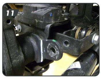
Install the shorter passenger side post on the side of the track bar mount at the sway bar link mount location with it pointing outboard [12]. Fasten with the ½" nylock nut and tighten to 65 ft-lbs.
