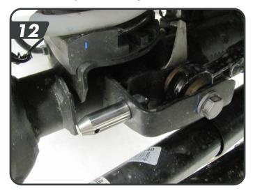
w. Install the longer disconnect post on the driver side axle sway bar link mount with it pointing inboard [13]. Fasten with the ½" nylock nut and tighten to 65 ft-lbs. Tighten the post with the pin hole parallel to the ground. Slide the polyurethane spacer on the pin up against the axle tab.
