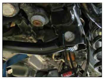
O Loosely install the original mounting hardware.
