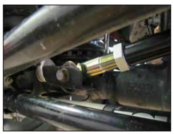
O Double check the axle center measurment and readjust if necessary.
