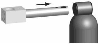
O Slide remaining Mounting Block (B) onto opposite end of Cross Pin (A), making sure bolt and roll pin holes are correctly positioned.
