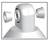
**HINT:** Position Conical Spacers with narrow ends facing spherical bearing.
