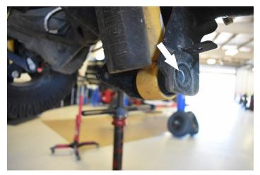
O While the strut is held forward for the hole to align, slide the skid plate over the mounting bracket and install 2 of the provided M20 washers from bolt pack J168 (one on each side) between the skid plate and factory bracket as shown below.
