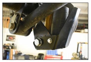
• Using the JKS badges and the supplied rivets in bolt pack 887 install the JKS badges on the rear of your skid plates as shown below.
