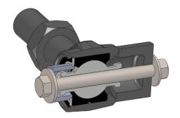
O Place the large nylon cup on the end that will not have the snap ring removed with the cupped end towards the flex eye as shown.
